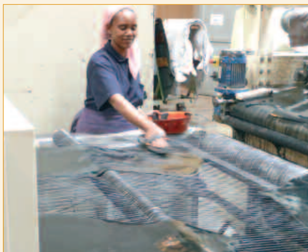
Patch-padding after roller coating.
