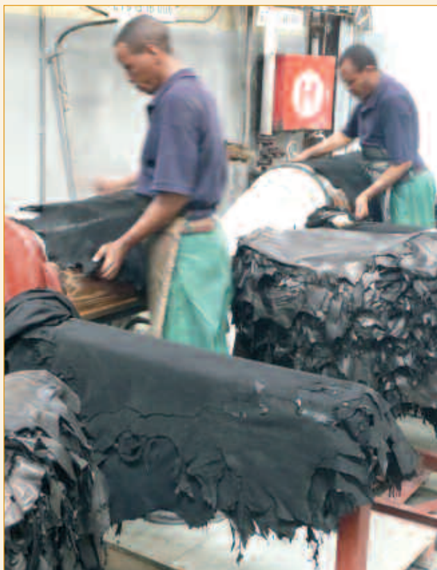
Final hand polishing operation.
