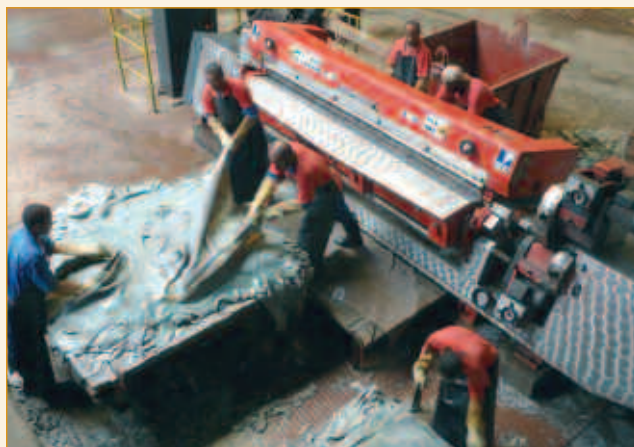
Lime splitting team. Trimmings and thin limed splits are sold for rendering.
