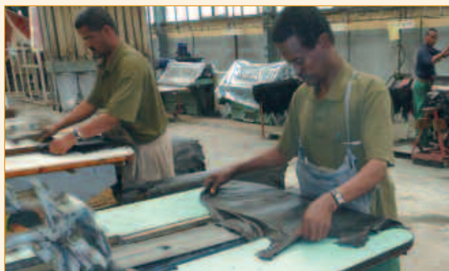
Hand staking for ultimate softening.
