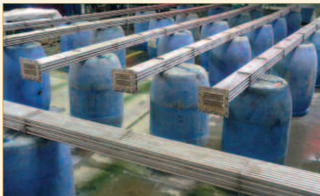
Heat exchangers from within a vacuum drying unit undergoing in-house maintenance.
