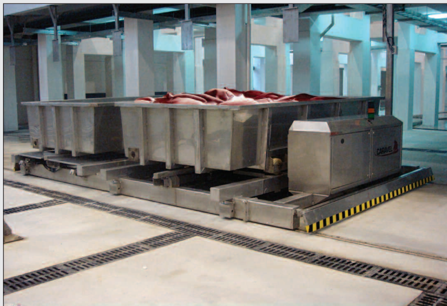
Rationalising the movement of wet dyed leathers: The automatic guided vehicle carrying two containment vessels.
