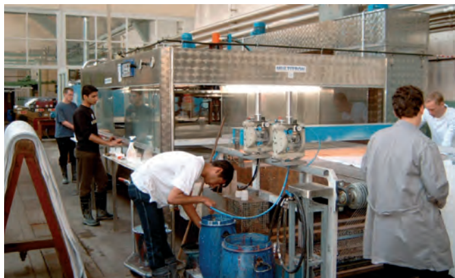
The finish spraying line at LGR
