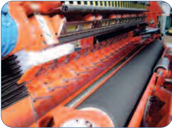
View across the splitting machine in the open position showing the opened jaw plate assembly. The knife is removed.
