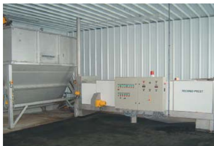
Salt recovery unit with a capacity of 500 tons per year
