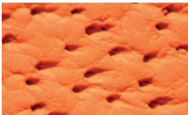
Panel 7: Full grain crust observed by light microscope
