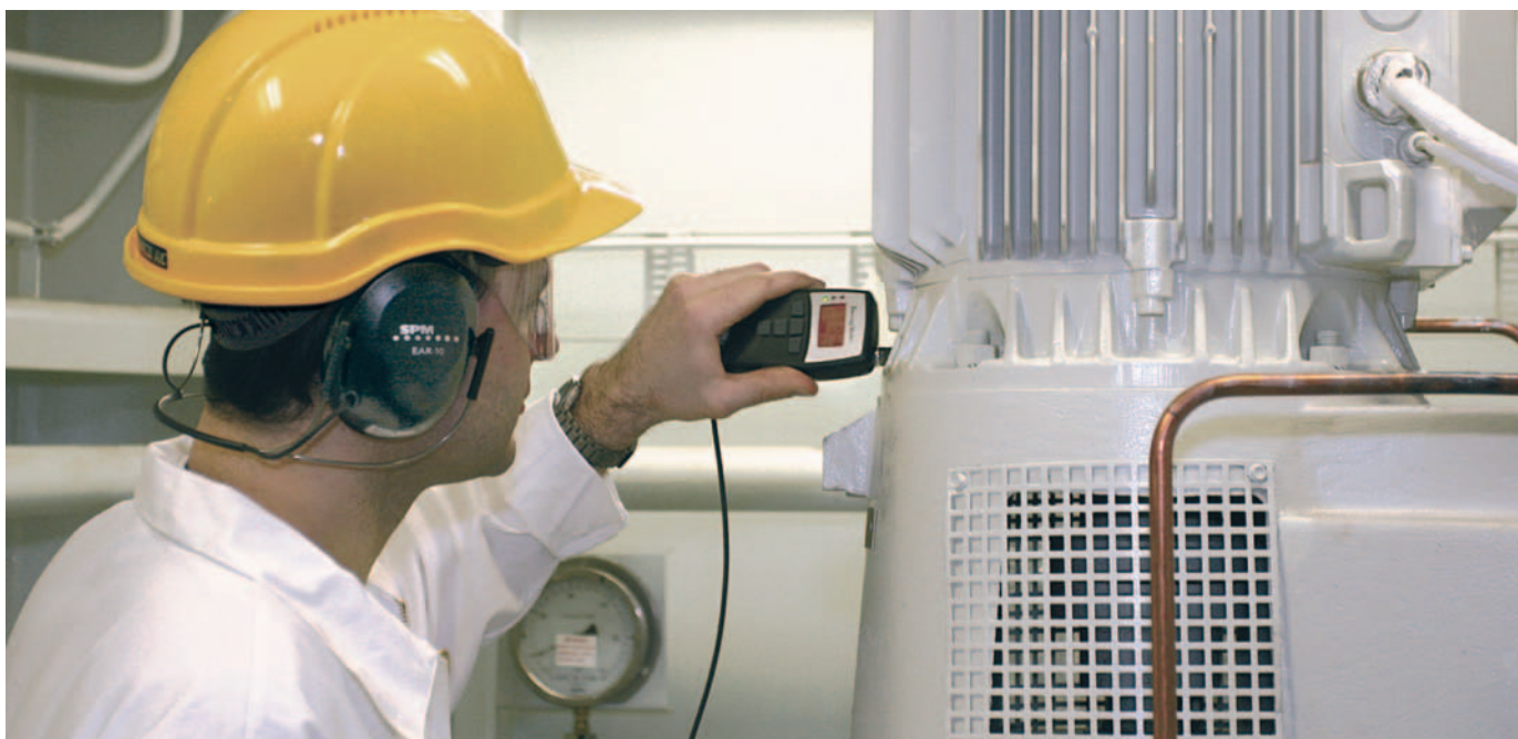
Predictive maintenance involves regular scheduled and detailed inspection of a running machine (SPM Instrument)
