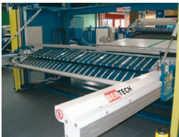
Figure 1: Persico's throughfeed fleshing machine—still the market leader
