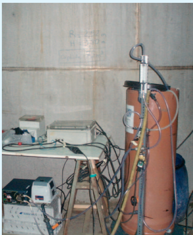
Left to right: Process control unit, peristaltic pump, blower and bioreactor
