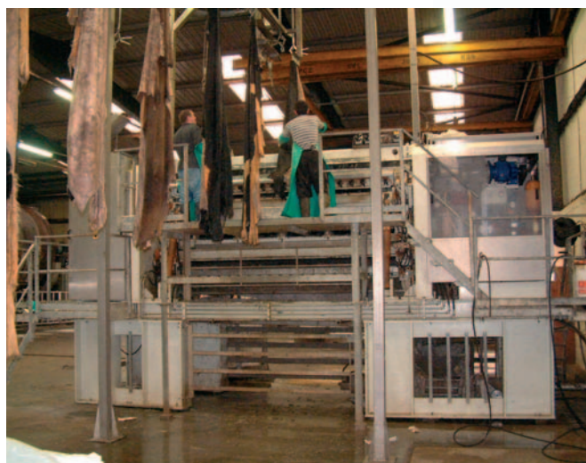
Persico "Perscarma" throughfeed flesher fed by overhead chain conveyor
