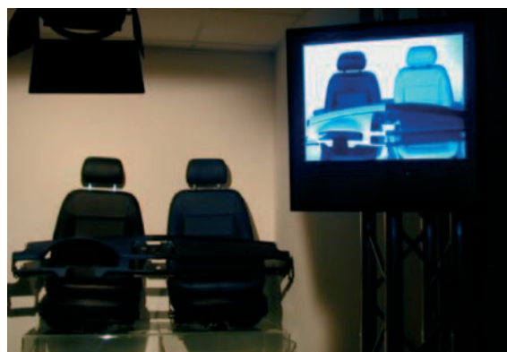
(b) Black and white IR image of Cool and non-Cool car seats and dashboard. The cool car seat and dash board appears in light colour as it reflects NIR waves.
