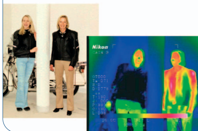
Panel 6: IR image made from black motorbike leather (Cool on the left and non-Cool on the right side)
