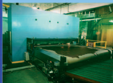
The world's biggest hydraulic press for leather. Capacity 4.000 t for 180 hides p/h
