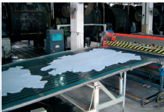
...and are delivered to the infeed conveyors of the Diamond splitter
