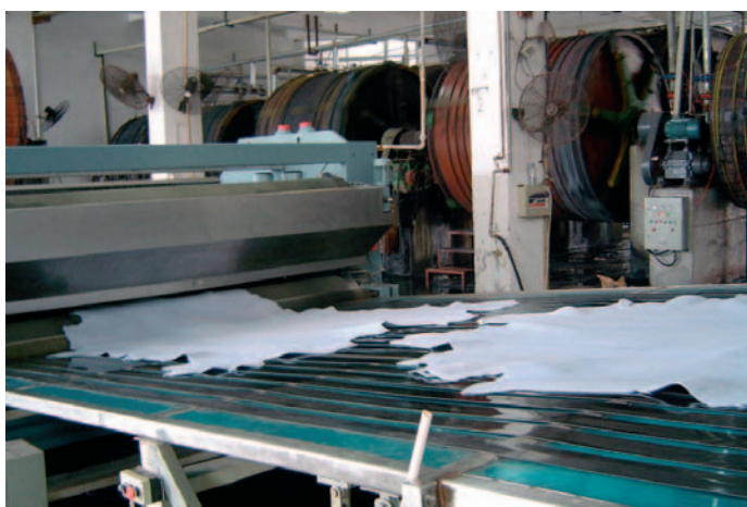
Hides leave the Bauche throughfeed samm/setting flat and unpleated...
