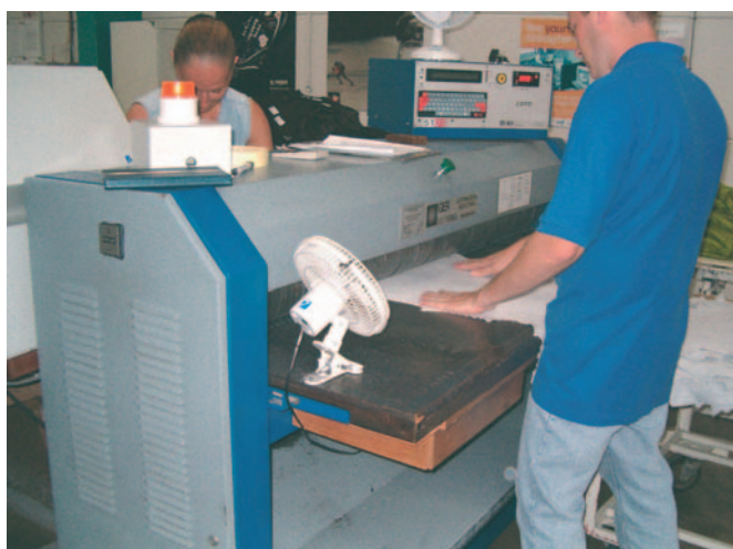
Photo-electric measurement of area was the first real application of computer technology in the tannery
