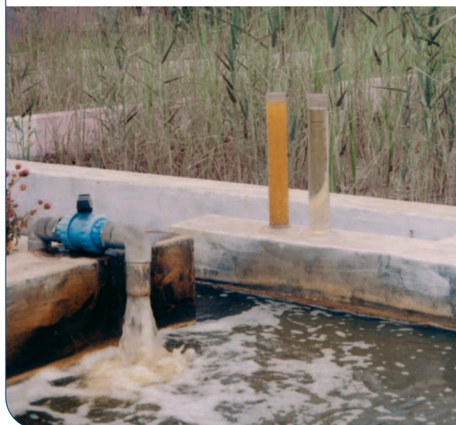
Panel 1: Example of a tannery effluent before and after reedbed treatment
