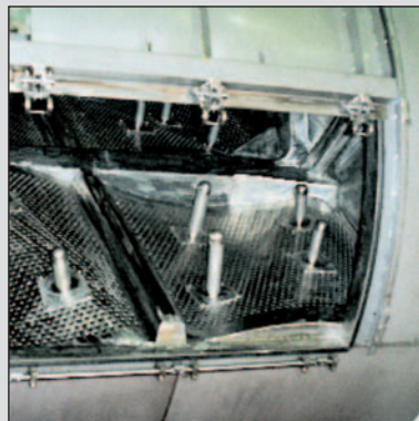
Compartmental design combining shelf profiling and pegs.
