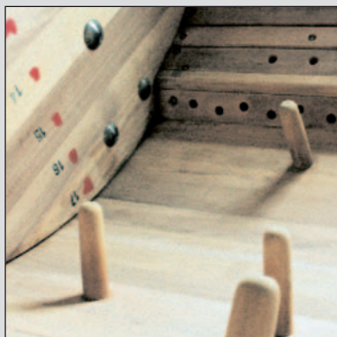
Shelves in a drum (perforated for recirculation) combined with pegs.
