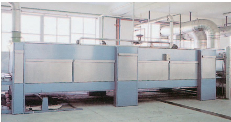
A conventional steam-heated drying tunnel (Tecnolettro)
