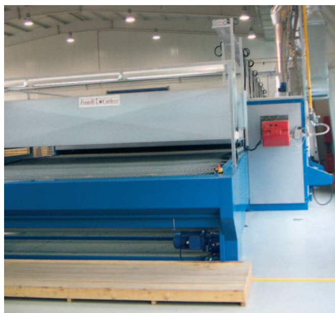
Another design of a gas-fired tunnel with burner mounted to one side (Carlessi)
