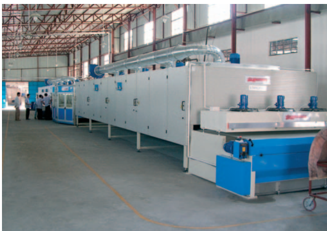
A large modern steam drying tunnel from Gemata
