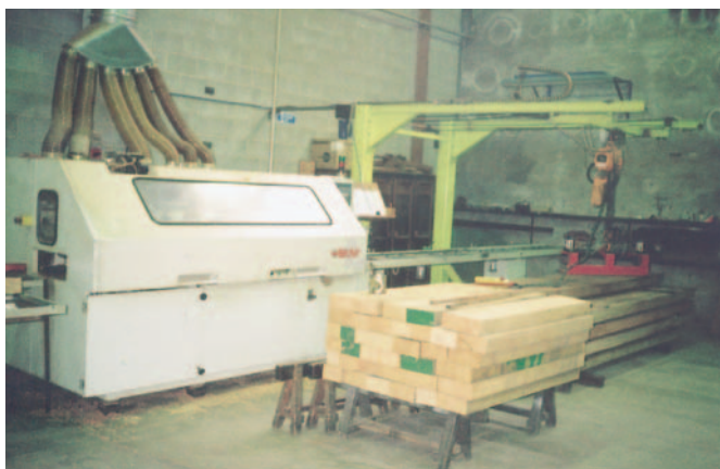
Figures 2 & 3: C.N.C. machining centres shape timber into precision components
