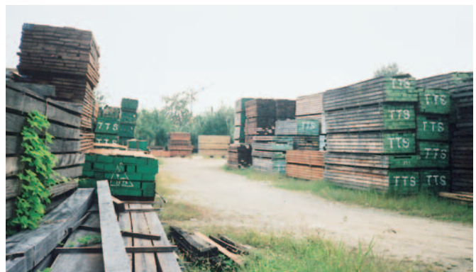
Figure 1: Timber for three years of production stacked for seasoning outside the factory
