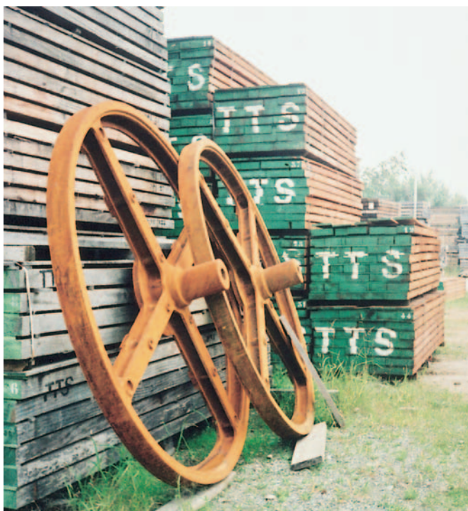
Figure 4: Crown wheel castings seasoning outside before machining
