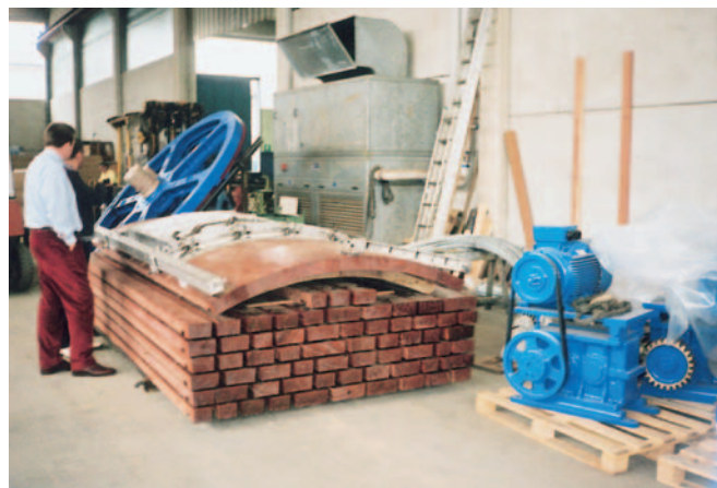
Figure 6: Pre-fabricated drum door section and staves await packing for despatch
